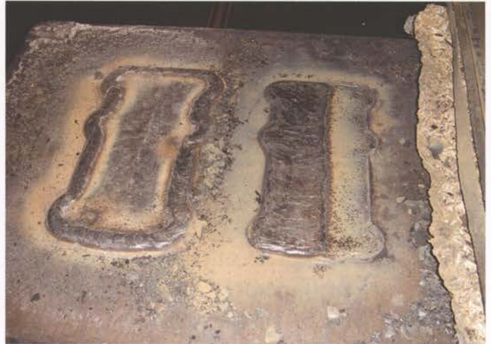
Figure 3. Flood-welded press die ready for machining.
